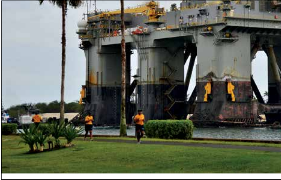
Sea-based X-band radar, world's largest phased-array X-band radar carried aboard mobile, ocean-going semisubmersible oil platform, transits waters of Joint Base Pearl Harbor–Hickam (U.S. Navy/ Daniel Barker)
